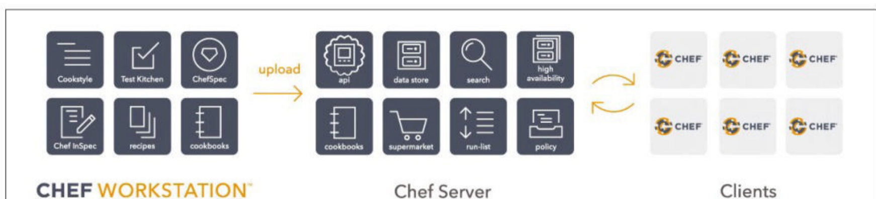
Figure 4: Chef Infra comprises the server, the client, and the workstation. It is joined by the InSpec compliance tester with the Habitat CI/CD tool. © Chef
